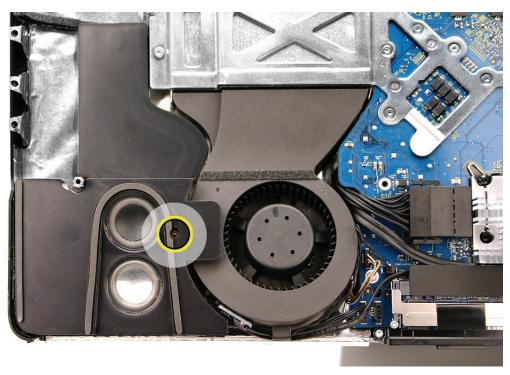
2. Route the speaker cable under the cable clip on the CPU fan and under the long cable guide above the memory slots. Connect the speaker cable to the audio board on the right side.
